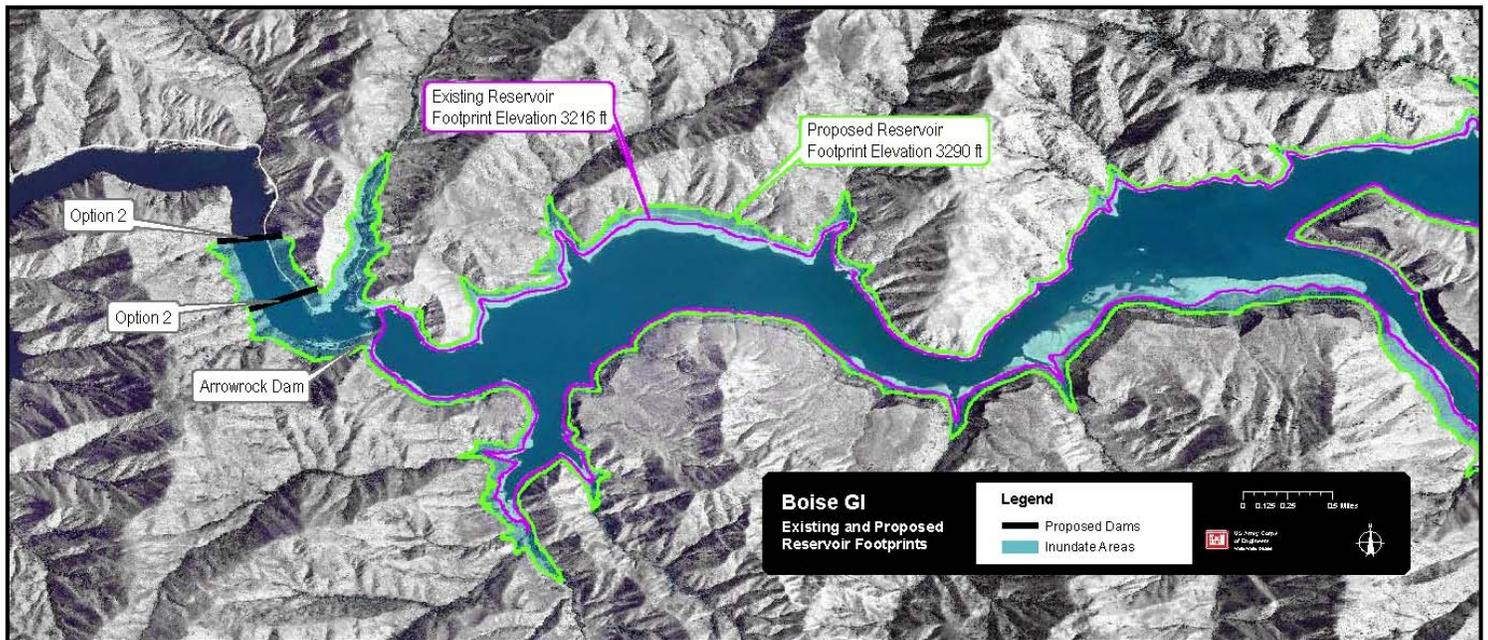
**Plan view showing conceptual reservoir footprints for expanded Arrowrock Reservoir capacity through a dam raise or a new dam constructed downstream (Options 1 or 2). The green line shows the increased reservoir boundary. Approximately 6.5 miles of additional river would be inundated with a dam raise.**
